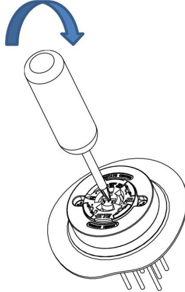
Figure 8 Use screwdriver to turn the center housing to the desired position.
